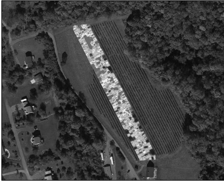
GPR data from Chester Gap Cellars in Rappahannock County. Map reflects an average of subsurface properties down to about 5 feet bgs. Red represents areas with a high dielectric constant, blue represents areas with a low dielectric constant. Red areas may represent subsurface “reflectors” of the GPR signal (e.g. rocks or clay pockets.)
