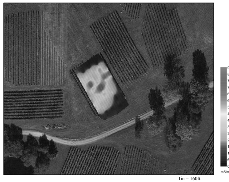
Figure 21 - EM conductivity map from an all-steel block at Linden Vineyards in Fauquier County. Overprint seen to mask soil EC variations here as well. A wide range of conductivity values is noted.
