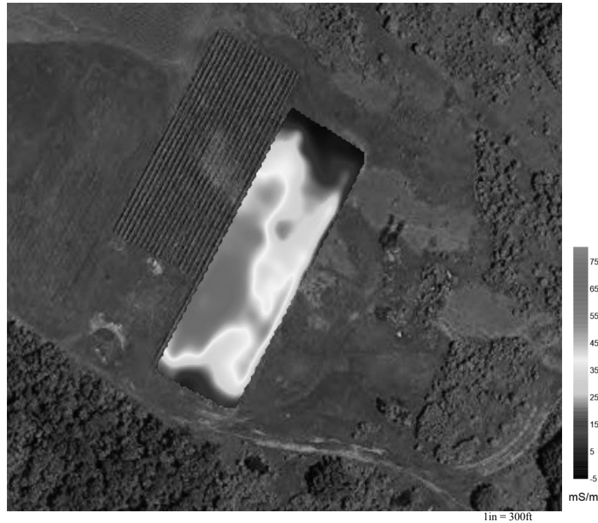
Figure 22 – EM conductivity map from an all-steel vineyard in Albemarle County, Virginia. A wider row spacing makes for a more useful EM38 dataset in this steel vineyard block as correlations to soil properties were noted; however, the overprint of the steel noise is still apparent on the map and may mask important soil EC variations. A wide range of conductivity values is seen here as well.
