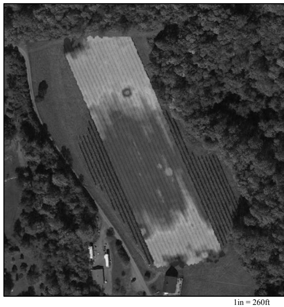
Figure 18 - EM conductivity map from Chester Gap Cellars, Rappahannock County. Classic steel vineyard overprint (low on the north and south ends, high in the middle) masking variations in soil EC.
