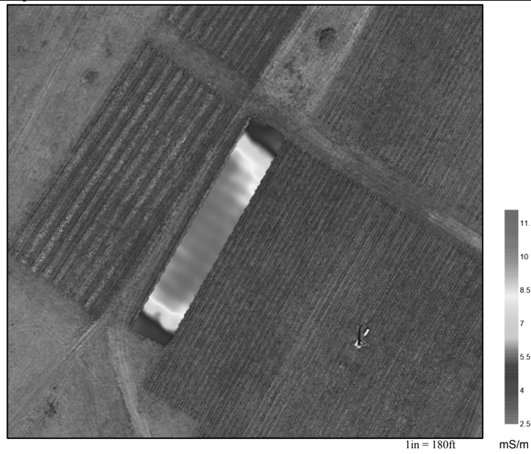
Figure 20 - Familiar overprint from steel trellising seen on EM conductivity map from an all-steel vineyard at Early Mountain Vineyards in Madison County. Any variations in subsurface conditions are masked by the noise created from the all-steel trellising.
