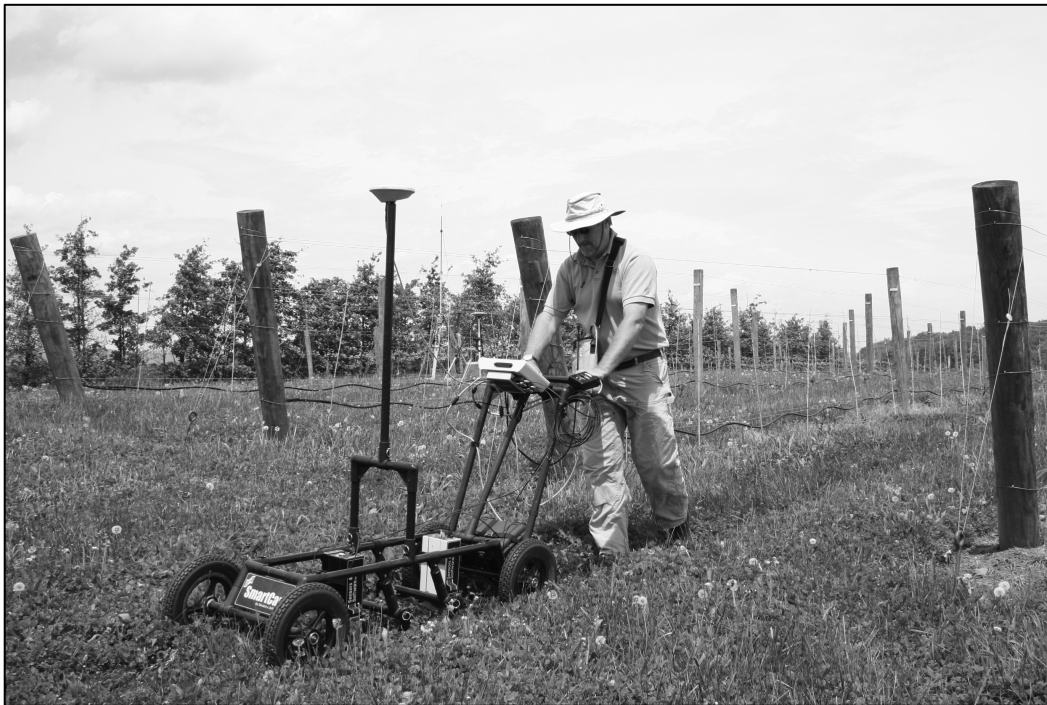
The field worker pushes the GPR cart along parallel profile lines during data collection; the lines are later integrated to produce plan view maps of the GPR data.
