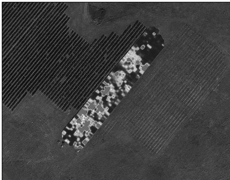
GPR data from Mt. Juliet Farm in Albemarle County. Red colors represent areas with a high dielectric constant, blue represents areas with a low dielectric constant. This map represents subsurface properties down to about 5 feet bgs. Red areas may represent subsurface “reflectors” of the GPR signal here as well (e.g. rocks or clay pockets).
